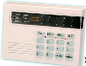
The DMP 692 Security Command® is a highly attractive, user-friendly LED keypad with three optional 2-button Panic keys. Sixteen LEDs on the 692 include three system status LEDs, three armed status LEDs, and ten zone LEDs. The 692 also includes an easy-to-read backlit keyboard, simple COMMAND key arming, and a built-in alert buzzer. The 692 is encased in a stylish and durable plastic housing with removable base for easy installation.
